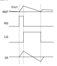
In SLLM (SLLM=0V), SLLM function is operated when LG pin is OFF and the coil current is lower than 0A (the current goes from Vout to SW). And it stops to output next HG.
