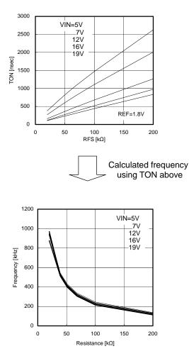
On Time (TON) at steady state is determined by resistance value connected to FS pin as shown in the figure. The frequency can be calculated with TON, input voltage VIN, the reference voltage REF as follows.
