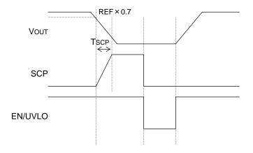
Short protection kicks in when output falls to or below REF X 0.7. When the programmed time period elapses, output is latched OFF to prevent destruction of the IC. Output voltage can be restored either by reconnecting the EN pin or disabling UVLO. Short circuit protection time is programmed using formula (4) below.
