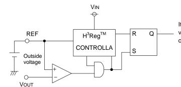
It is available to synchronize setting the reference voltage (REF) with outside supply voltage [V] by using outside power supply voltage.
