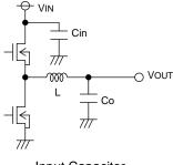
The input capacitor selected must have low enough ESR resistance to fully support large ripple output, in order to prevent extreme over current. The formula for ripple current IRMS is given in (10) below.
