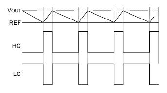
When Vout falls to a threshold voltage (REF), the drop is detected, activating the  $H^3Reg^{TM}$  CONTROLLA system.
