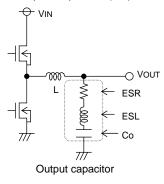
series resistance required to smooth out ripple volume and maintain a stable output voltage range.
