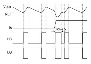
When VOUT drops due to a rapid load change, and the voltage remains below REF after the programmed TON time interval has elapsed, the system quickly restores VOUT by extending the TON time, improving the transient response.
