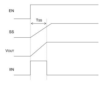
Soft start is exercised with the EN pin set high. Current control takes effect at startup, enabling a moderate output voltage "ramping start." Soft start timing and incoming current are calculated with formulas (2) and (3) below.
