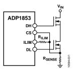
Figure 25. Accurate Current-Limit Sensing
