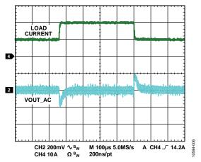
Figure 5. 10 A to 20 A Load Step,  $12\,V_{\rm IN}$  to 3.3  $V_{\rm OUT}$ , 300 kHz, Current Mode
