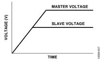
Figure 31. Coincident Tracking
