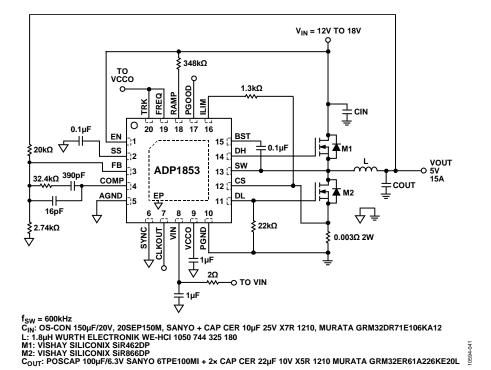
Figure 35. 15 A Circuit Operating in Current Mode
