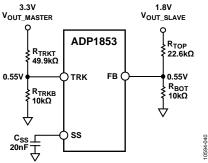
Figure 34. Example of a Ratiometric Tracking Circuit
