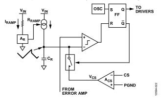
Figure 16. Simplified Control Architecture
