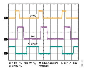
Figure 10. Synchronization and CLKOUT,  $f_{SYNC} = 300 \text{ kHz}$
