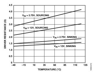
Figure 15. Driver Resistance vs. Temperature
