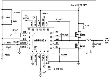
f<sub>SW</sub> = 300kHz C<sub>IN</sub>: OS-CON 150μF/20V, 20SEP150M, SANYO + CAP CER 10μF 25V X7R 1210, MURATA GRM32DR71E106KA12 L: 1μH COILCRAFT SER1412-102ME M1: INFINEON BSC052N03LS M2: INFINEON BSC0902NS
