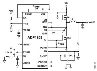
Figure 1. Typical Operation Circuit
