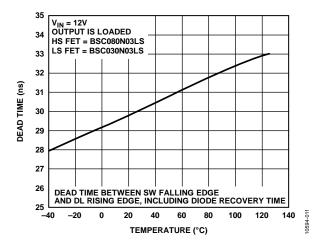
Figure 11. Dead Time vs. Temperature
