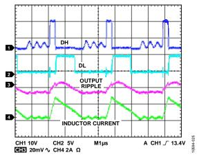
Figure 19. Example of Discontinuous Conduction Mode (DCM) Waveform
