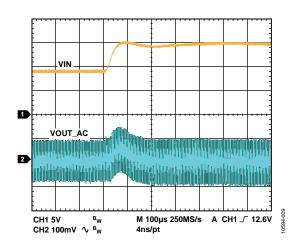
Figure 9. 9 V to 15 V Line Step, 3.3 V<sub>OUT</sub>, 15 A Load, Voltage Mode
