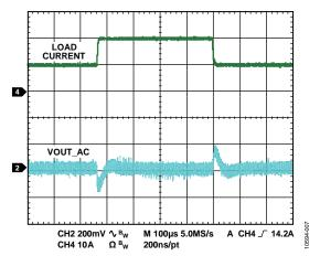
Figure 8. 10 A to 20 A Load Step,  $12\,V_{\rm IN}$  to 3.3  $V_{\rm OUT}$ , 300 kHz, Voltage Mode
