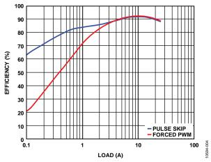
Figure 4. Efficiency Plot 12  $V_{\rm IN}$  to 3.3  $V_{\rm OUT}$ , 300 kHz, see Figure 36 for Circuit
