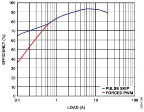
Figure 7. Efficiency Plot 15  $V_{\rm IN}$  to 5  $V_{\rm OUT}$ , 600 kHz, see Figure 35 for Circuit
