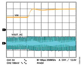
Figure 6. 9 V to 15 V Line Step, 3.3 V<sub>OUT</sub>, 15 A Load, Current Mode
