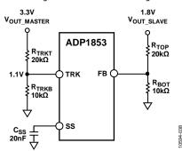
Figure 32. Example of a Coincident Tracking Circuit
