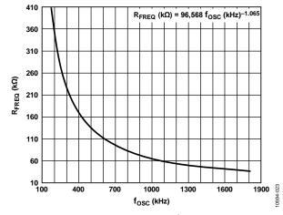
Figure 17.  $R_{FREQ}$  vs.  $f_{OSC}$
