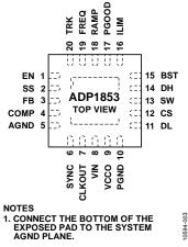
Figure 3. Pin Configuration
