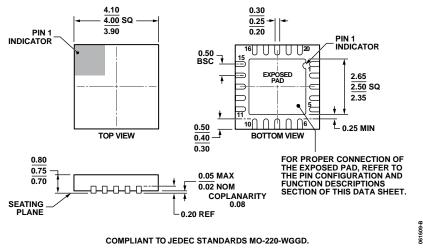
Figure 37. 20-Lead Lead Frame Chip Scale Package [LFCSP\_WQ] 4 mm × 4 mm Body, Very Very Thin Quad (CP-20-10) Dimensions shown in millimeters
