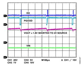
Figure 21. Overvoltage Protection in PSM
