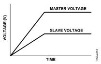
Figure 33. Ratiometric Tracking
