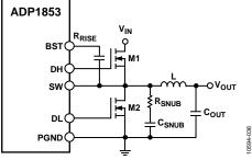
Figure 30. Application Circuit with a Snubber
