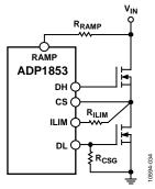
Figure 28. Slope Compensation and CS Gain Connection
