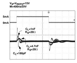
FIGURE 4. TRANSIENT LOAD REGULATION (SINKING)
