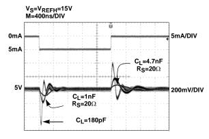
FIGURE 3. TRANSIENT LOAD REGULATION (SOURCING)
