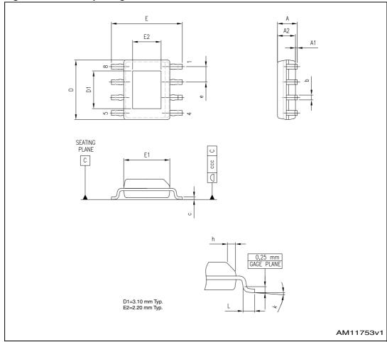
Figure 38. HSOP8 package dimensions
