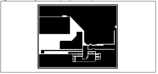
Figure 20. PCB layout: A7986A (bottom side)
