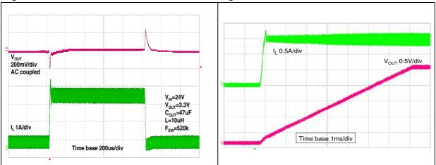
Figure 32. Short-circuit behavior V<sub>IN</sub>=12 V Figure 33. Short-circuit behavior V<sub>IN</sub>=24 V
