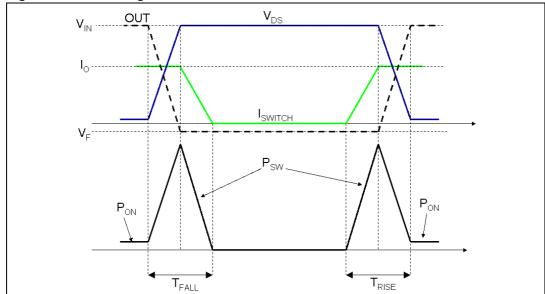
Figure 16. Switching losses
