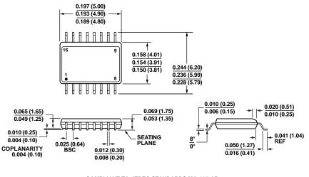
COMPLIANT TO JEDEC STANDARDS MO-137-AB CONTROLLING DIMENSIONS ARE IN INCHES; MILLIMETERS DIMENSIONS (IN PARENTHESES) ARE ROUNDED-OFF INCH EQUIVALENTS FOR REFERENCE ONLY AND ARE NOT APPROPRIATE FOR USE IN DESIGN.
