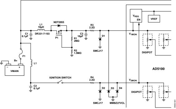
Figure 19. Protection Circuits
