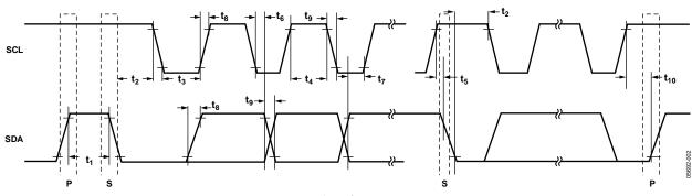
Figure 2. Digital Interface Timing Diagram
