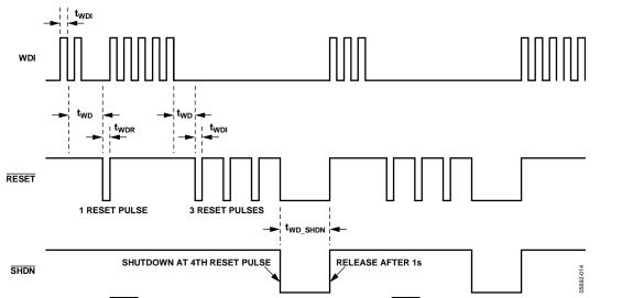
Figure 14. Advanced Watchdog—SHDN Asserted After Three Trials of Resetting the Watchdog (SHDN Released After 1 Second and the Cycle Repeats)
