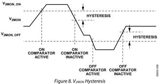
By default,  $V_{2MON}$  is level sensitive and the on and off thresholds are both monitored. The on threshold chosen must be greater than the off threshold.
