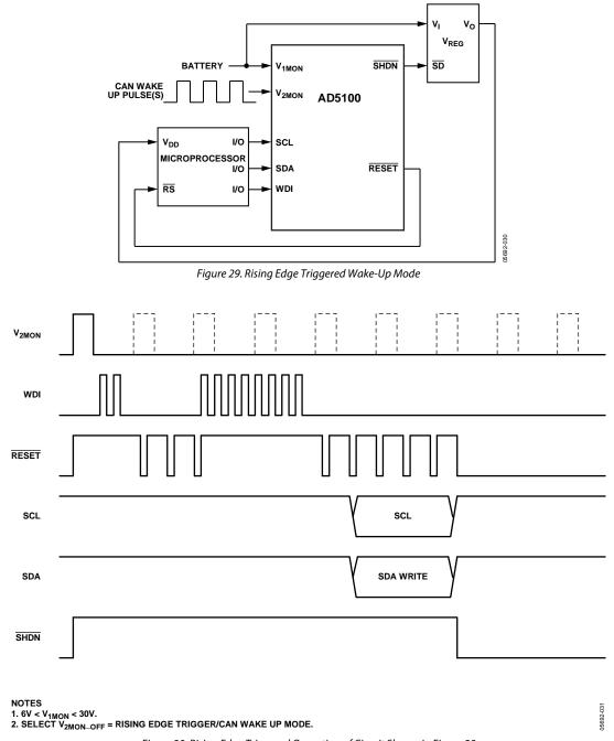
Figure 30. Rising Edge Triggered Operation of Circuit Shown in Figure 29
