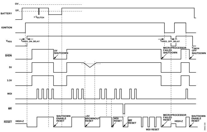
Figure 25. Example of SHDN and RESET Responses of Circuit Shown in Figure 24
