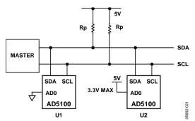
Figure 20. Two AD5100 Devices on One Bus
