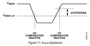
The V<sub>4MON</sub> comparator is used to control the V<sub>4OUT</sub> pin and (in conjunction with a hold timer) to control the RESET pin. To configure V<sub>4MON</sub> to control the RESET pin, set Register 0x0D[3] to 0. Setting this bit to 1 prevents V<sub>4MON</sub> from causing RESET to activate. The default setting is V<sub>4MON</sub> does not cause RESET to activate.
