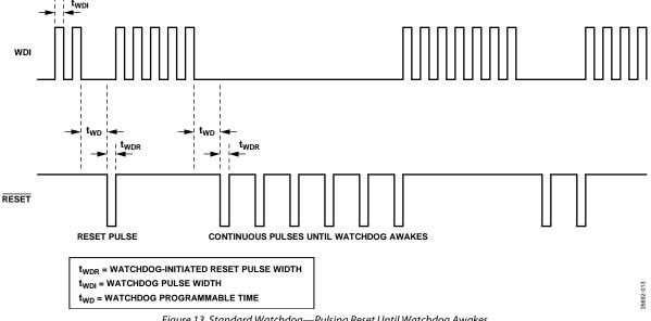
Figure 13. Standard Watchdog—Pulsing Reset Until Watchdog Awakes
