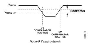
The  $V_{3MON}$  comparator is used (in conjunction with a hold timer) to control the RESET pin.
