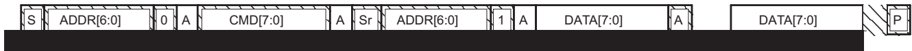
Figure 7. Supported I2C formats : (a) 1-byte write; (b) quick read; (c) 1-byte read; (d) incremental read
