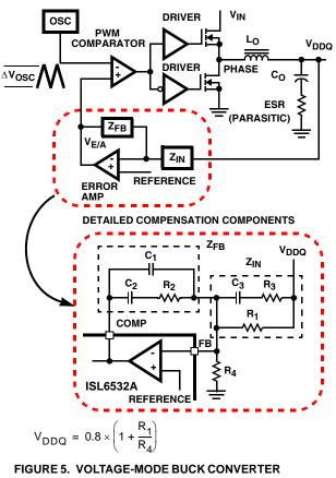
FIGURE 5. VOLTAGE-MODE BUCK CONVERTER COMPENSATION DESIGN AND OUTPUT VOLTAGE SELECTION
