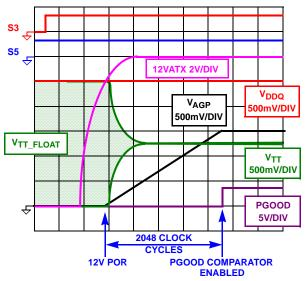
FIGURE 2. TYPICAL S3 to S0 STATE TRANSITION
