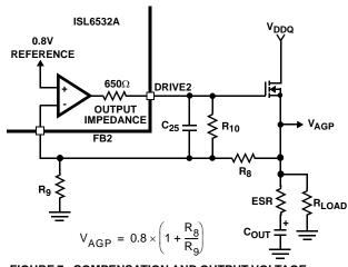
FIGURE 7. COMPENSATION AND OUTPUT VOLTAGE SELECTION OF THE LINEAR
