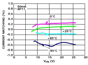
FIGURE 8. CURRENT MATCHING vs V<sub>IN</sub> vs TEMPERATURE
