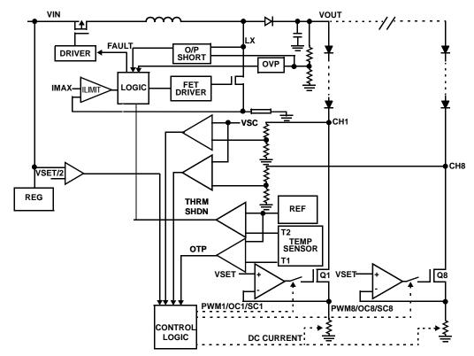
FIGURE 25. SIMPLIFIED FAULT PROTECTIONS
