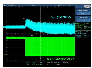
FIGURE 20. LOAD REGULATION WITH I  $_{\rm LED}$  CHANGES FROM 100% TO 0.4% PWM DIMMING
