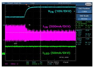
FIGURE 17. LINE REGULATION WITH  $V_{1N}$  CHANGES FROM 12V TO 26V DISABLE PROFILE
