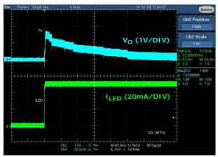
FIGURE 21. LOAD REGULATION WITH I<sub>LED</sub> CHANGES FROM 0% TO 100% PWM DIMMING
