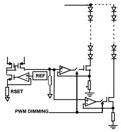
FIGURE 24. SIMPLIFIED CURRENT SOURCE CIRCUIT
