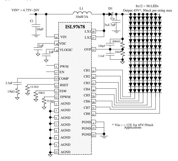
FIGURE 1. ISL97678 TYPICAL APPLICATION DIAGRAM
