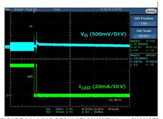
FIGURE 22. LOAD REGULATION WITH I<sub>LED</sub> CHANGES FROM 100% to 0% PWM DIMMING
