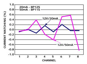
FIGURE 7. CHANNEL-TO-CHANNEL CURRENT MATCHING EXAMPLE
