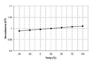
Figure 13. LV<sub>CC</sub> OVP Voltage vs. Temperature
