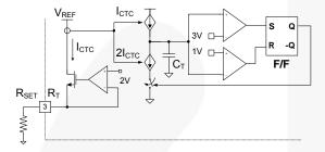
Figure 17. Current Controlled Oscillator
