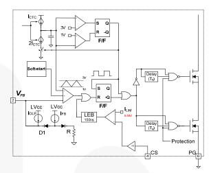
Figure 19. Internal PWM Block Diagram
