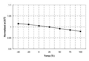
Figure 7. High-Side  $V_{CC}$  (HV<sub>CC</sub>) Start vs. Temperature Figure 8. High-Side  $V_{CC}$  (HV<sub>CC</sub>) Stop vs. Temperature
