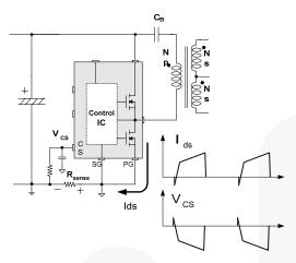
Figure 21. Half-Wave Sensing
