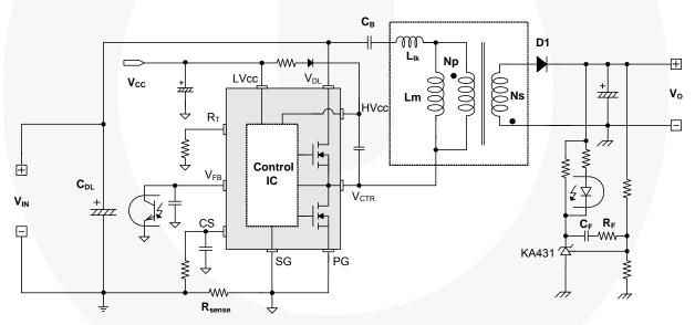
Figure 2. Typical Application Circuit for an Asymmetric PWM Flyback Converter
