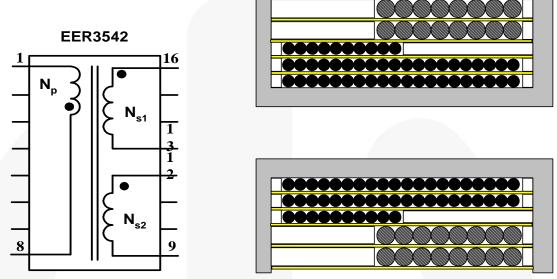
Figure 27. Core and Winding
