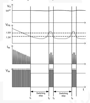
Figure 25. Burst-Mode Operation
