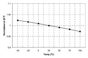
Figure 5. Maximum Duty Cycle vs. Temperature
