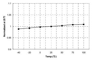
Figure 11. OLP Delay Current vs. Temperature
