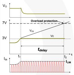
Figure 23. Overload Protection
