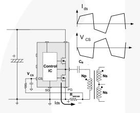
Figure 22. Full-Wave Sensing
