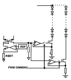
FIGURE 24. SIMPLIFIED CURRENT SOURCE CIRCUIT
