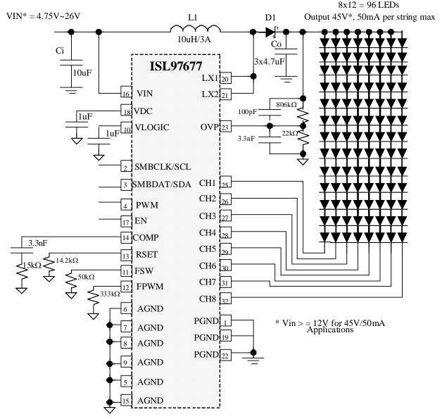
FIGURE 1. ISL97677 TYPICAL APPLICATION DIAGRAM
