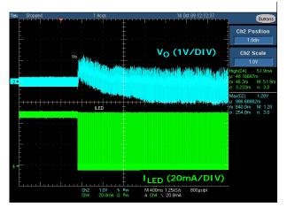
FIGURE 20. LOAD REGULATION WITH I $_{\rm LED}$  CHANGES FROM 100% TO 0.4% PWM DIMMING
