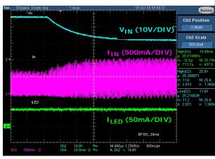
FIGURE 18. LINE REGULATION WITH  $V_{\mbox{\scriptsize IN}}$  CHANGES FROM 26V TO 12V
