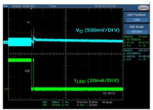
FIGURE 22. LOAD REGULATION WITH I<sub>LED</sub> CHANGES FROM 100% to 0% PWM DIMMING
