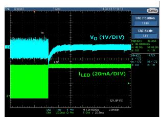
FIGURE 19. LOAD REGULATION WITH I<sub>LED</sub> CHANGES FROM 0.4% TO 100% PWM DIMMING
