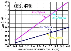
FIGURE 9. CURRENT LINEARITY vs LOW LEVEL PWM DIMMING DUTY CYCLE
