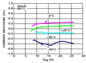
FIGURE 8. CURRENT MATCHING vs  $V_{IN}$  vs TEMPERATURE
