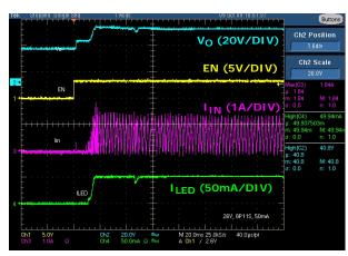
FIGURE 16. IN-RUSH CURRENT AND LED CURRENT AT  $V_{1N} = 26V$
