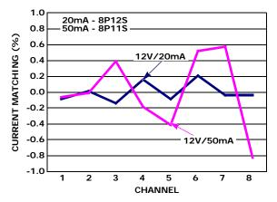
FIGURE 7. CHANNEL-TO-CHANNEL CURRENT MATCHING EXAMPLE
