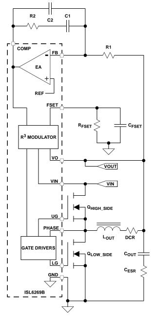
FIGURE 6. COMPENSATION REFERENCE CIRCUIT
