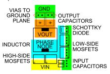
FIGURE 8. TYPICAL POWER COMPONENT PLACEMENT
