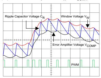
FIGURE 3. MODULATOR WAVEFORMS DURING LOAD TRANSIENT
