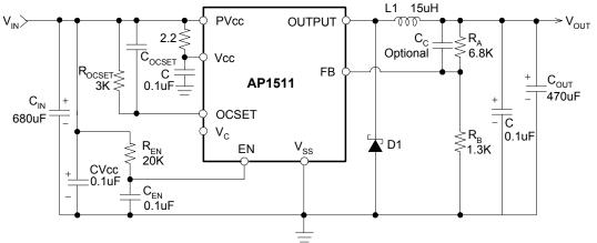
Note:  $V_{OUT} = V_{REF} x (1+R_A/R_B)$  $R_B = 1 K \sim 10 K \text{ ohm}$
