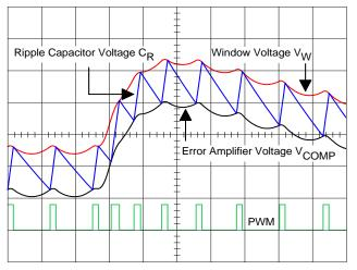
FIGURE 3. MODULATOR WAVEFORMS DURING LOAD TRANSIENT
