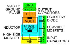
FIGURE 8. TYPICAL POWER COMPONENT PLACEMENT
