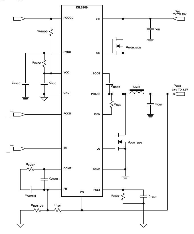
FIGURE 2. ISL6269 TYPICAL APPLICATION SCHEMATIC
