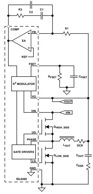
FIGURE 6. COMPENSATION REFERENCE CIRCUIT
