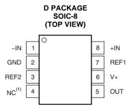
(1) NC: This pin is not internally connected. The NC pin should either be left floating or connected to GND.
