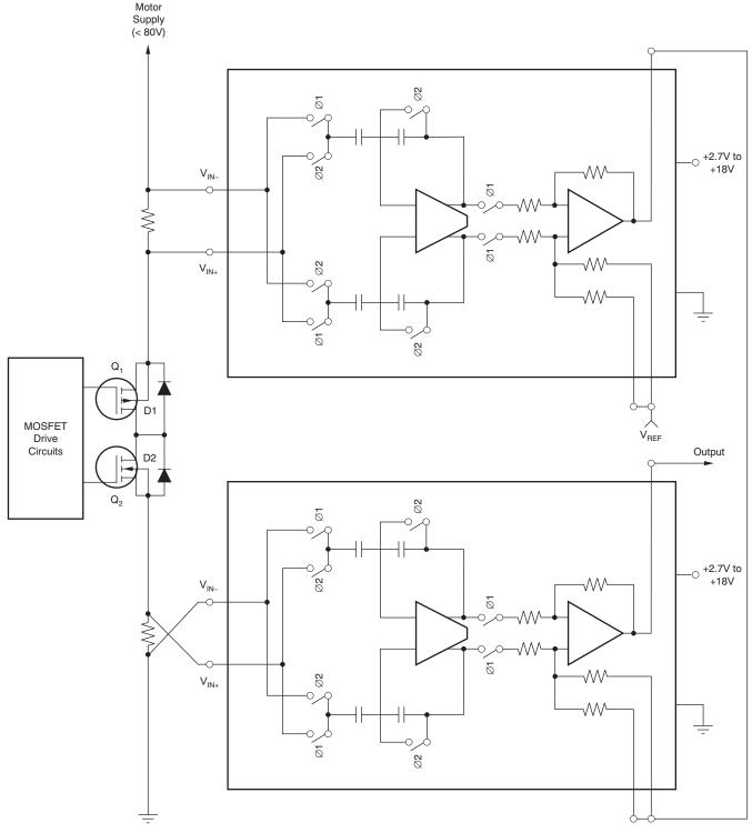
NOTE: By sensing totem-pole current on both the positive and negative rail and summing, dynamic common-mode issues can be avoided entirely. Note that IC<sub>2</sub> is connected with inverting inputs because it should report current with an opposite polarity to that of IC<sub>1</sub>.
