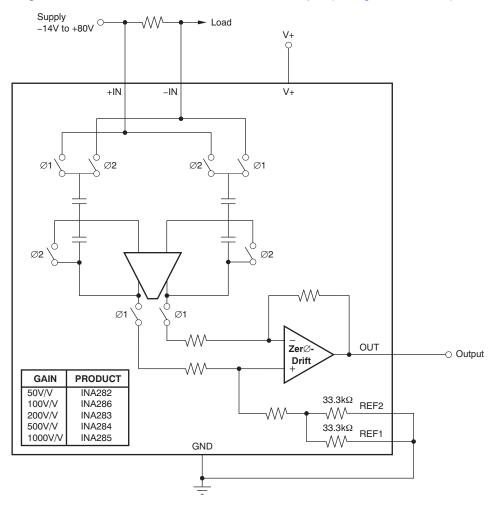
Figure 34. Ground Referenced Output
