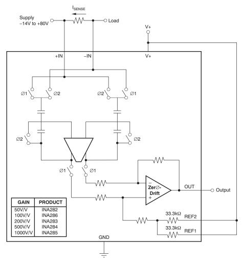
Figure 35. V+ Referenced Output
