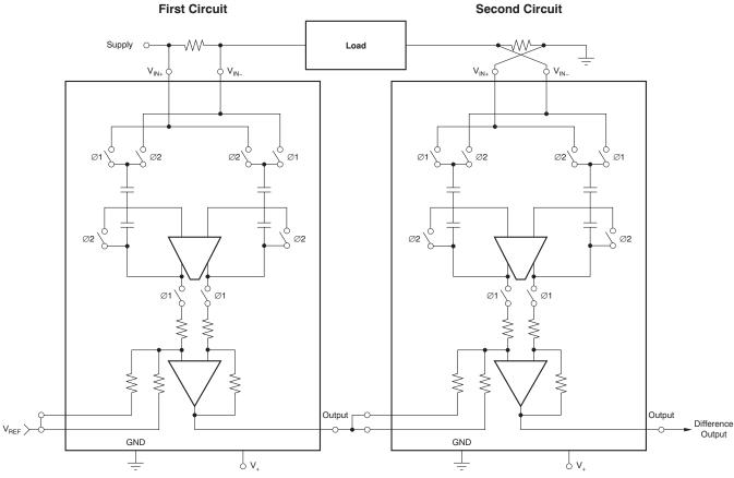
NOTE: This example is identical to the current summing example, except that the two shunt inputs are reversed in polarity, this current differencing circuit is useful in detecting when current into and out of a load do not match.
