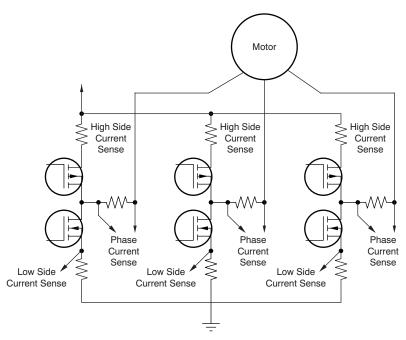
NOTE: Motor drive current sensing can be done on the low side, phase side, or high side. Only the phase output gives complete information regarding current in the motor, but is subject to common-mode transients that even the best amplifiers do not reject completely.
