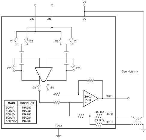
(1) Reference divider accuracy is determined by measuring the output with the reference voltage applied to alternate reference resistors, and calculating a result such that the amplifier offset is cancelled in the final measurement.
