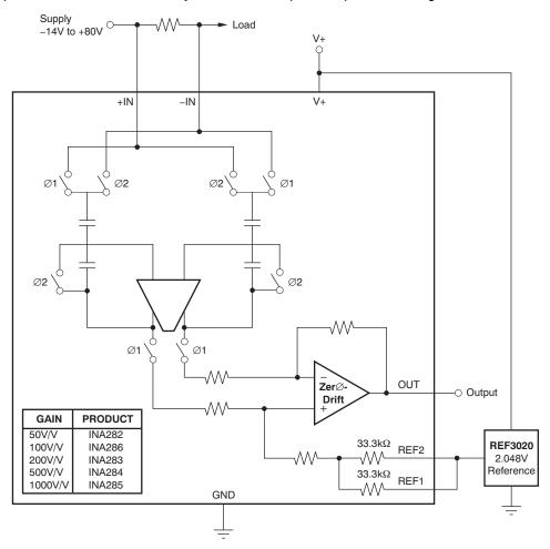
Figure 36. External Reference Output
