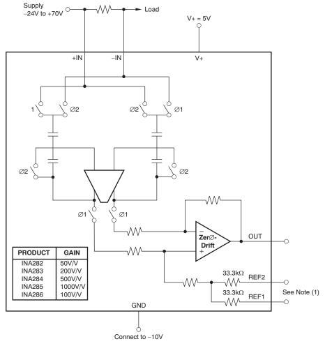
(1) Connect the REF pins as desired; however, they cannot exceed 9V above the GND pin voltage.
